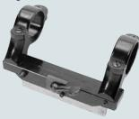
lock plunger to prevent accidental loss of removable part. Scope can be mounted low and be quickly removed for open sights or receiver sight. Low base only for bolt action rifles. Underside flat, no holes. Base must be prepared and installed by a gunsmith. Complete mount with 1" rings and blank base **J-200** Specify make and model of gun & scope when ordering.
