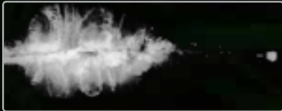
Simulated wound cavity in a gelatine block
